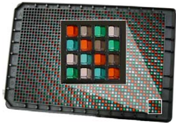
Figure 4: 1536-well reformatted plate. Inset is 4-well x 4-well close-up of dye dispense pattern.
