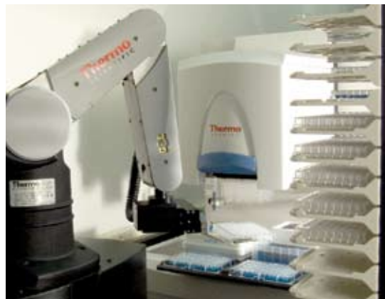
Figure 1: Catalyst Express robotic arm integrated with the Matrix PlateMate.
