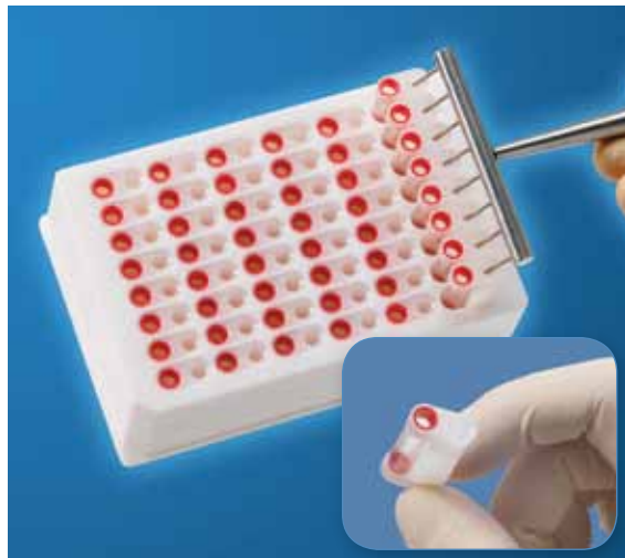
Figure 1: The Rapid Equilibrium Dialysis (RED) Apparatus. RED is composed of alternating rows of red cylindrical and white conical wells that are mutually linked to allow buffer entry into dialysis chamber.
